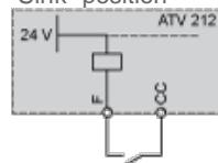
"PLC" position with PLC transistor outputs
